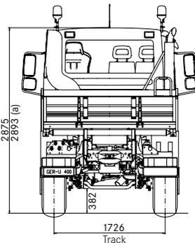
All dimensions in mm, shown with 365/80 R 20 tyres, (a) unladen, (b) with low platform intermediate frame, TC = trailer coupling
