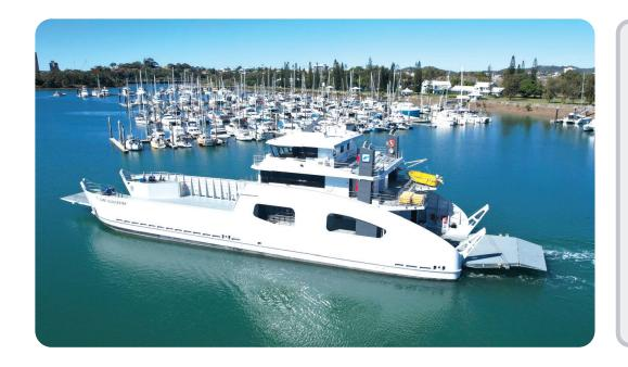
Cape Gloucester's impressive lines and styling give way to a capable work platform boasting 4.5m clearance under the accommodation deck.
