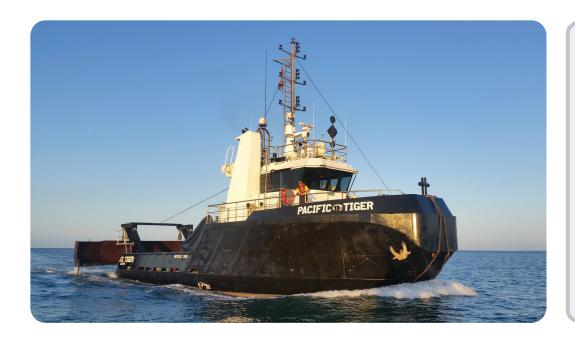
Pacific Tiger is a 24m twin-screw tug/utility vessel with a combined power rating of 1200hp and bollard pull of 15t.
