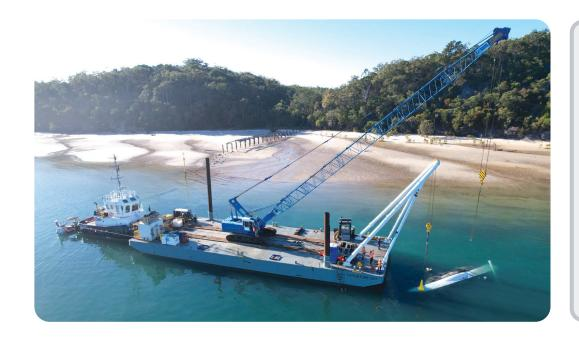
The Dumb Barge "Targetline 1201" measures 36m x 12m x 2.4m. Deck load capacity of 7t per square metre.
