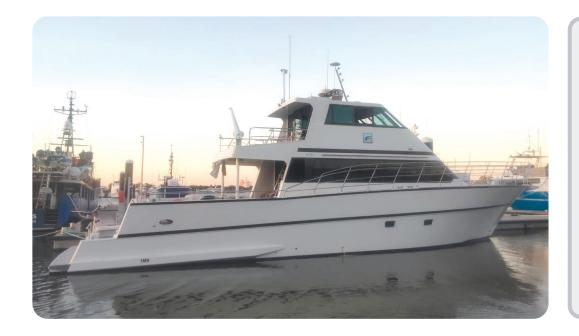
The Sounds Pacific is a versatile and comfortable 21m aluminium mono hull charter vessel.
