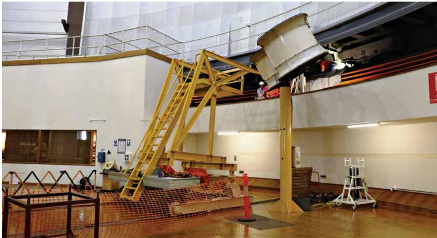
The 'bogie picker' could run on a trolley usually used to lift the optical telescope's mirror out for maintenance.
