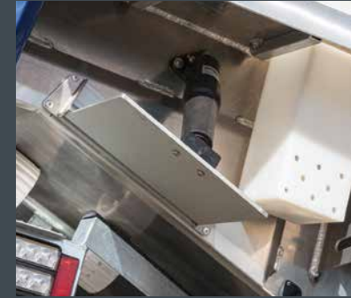
Trim tabs provide great side-to-side trim control for best performance
