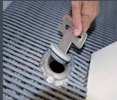
Easy-access fuel filler. Bar Crusher's fuel tank system has no leaky sub-floor hoses and you can see how much fuel you have left
