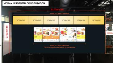
REMOVE EXISTING 6 SCREENS. APPLY BLACK MELAMINE TO WALL TO COVER CURRENT RECESS. HANG 12 SCREENS ON WALL USING BRACKETS AS PER THE ABOVE CONFIGURATION.
