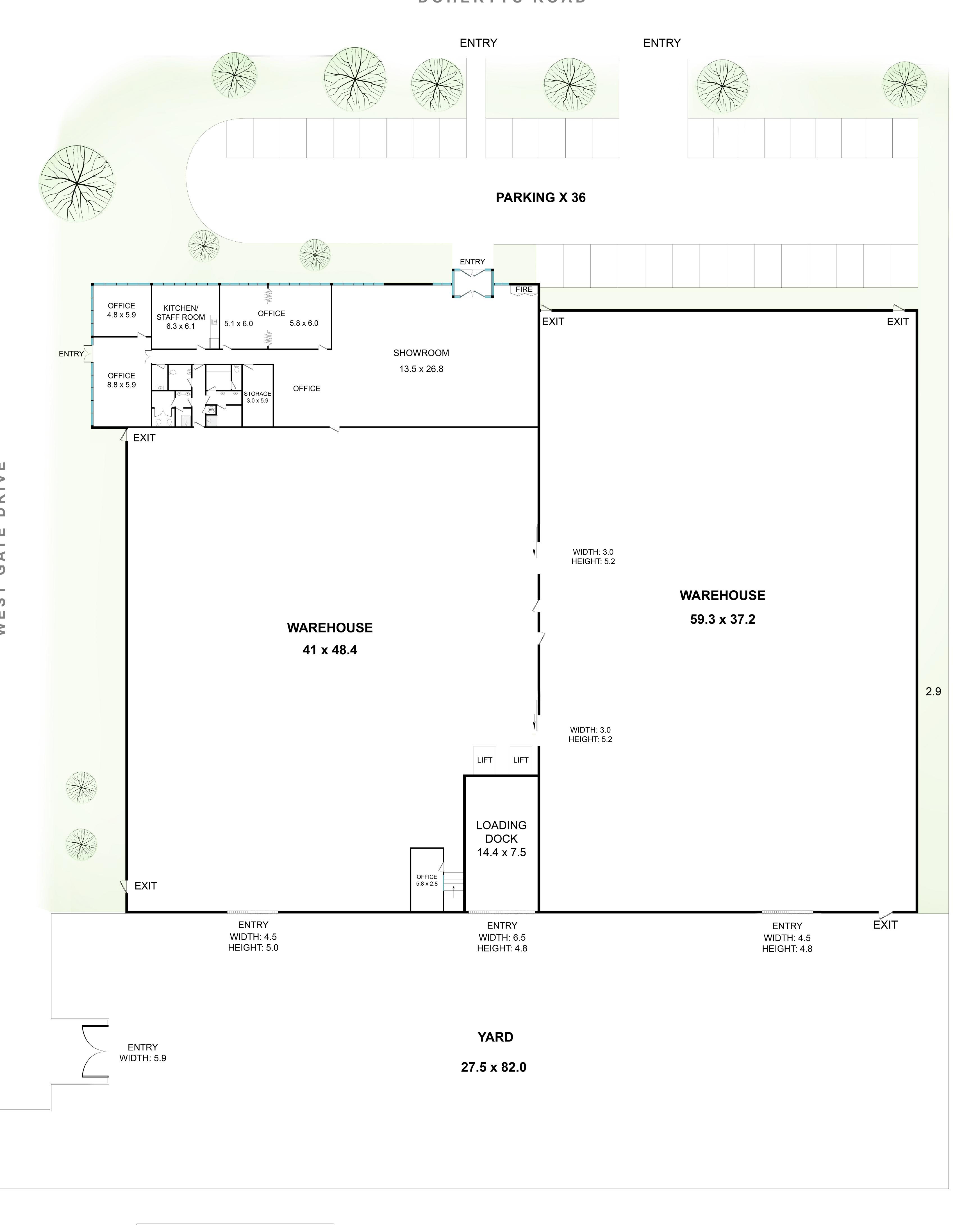
Warehouse ...  $4,292 \text{ m}^2$  Office/Showroom area ...  $590 \text{ m}^2$  Total building ...  $4,882 \text{ m}^2$  Storage yard ...  $2,519 \text{ m}^2$  Total site ...  $10,230 \text{ m}^2$
