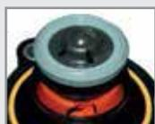
The diaphragm types are commonly known to rupture, especially when boost and temperature are increased as a result of chip tuning.
