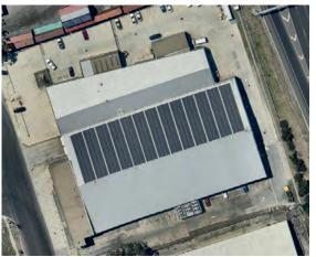
Already a highly efficient site, the addition of the 202 kW solar array has taken Tip Top's energy efficiency to a new level. The array was installed by Euan Angus Solar using LG panels and Fronius inverters, while Clean Technology Partners provided solar engineering services. LED lighting was also
