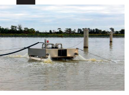
The aerator is assembled around a 2.2 kW submersible pump - the only moving parts of the system. Water is pumped through a specially designed manifold that directs it to each of four venturi injectors. Once the water and air have mixed, aerated water is ejected out of the nozzles positioned at each corner of the unit.
