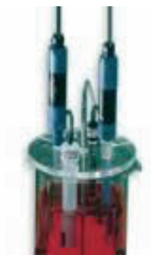
Measuring case for groundwater quality investigations, pH and ORP electrodes, conductivity probes
