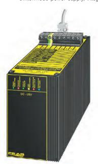
The UPS connects between the line voltage (85-270 VAC or 120-400 VDC) and the field equipment and is capable of supplying full load currents of up to 5 A at 24 VDC. To allow for intermittent high current demands upon the system, the full load current can be exceeded by up to 50% for limited periods of time. Additionally, the output is short-circuit and polarity protected to prevent damage caused by incorrect installation.
