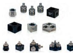
The hex and cube mounts are for traditional single-axis measurements. The tri-axial mount allows the user to select the same or different sensitivities on each orthogonal axis. For users that do not know the correct accelerometer sensitivity for the test, the tri-hex mount is suitable. The tri-hex mount allows the user to thread three different POD accelerometer sensor assemblies in a single mount.
