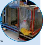
Solutions include: terminally mounted HEPA containment housings and systems; inline containment exhaust filtration systems; bag-in-bag-out (BIBO)-style containment systems with bubble-tight isolation dampers, decontamination/fumigation ports, a remote scan arrangement for testing and BIBO arrangements for filter change-out; customengineered HEPA (particulate) and HEGA (gaseous) containment filtration systems.
