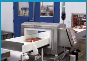
can be removed before reaching the metal detector. This arrangement can minimise the number of detections made by the metal detector, leading to fewer production disruptions and reduced loss of good products.
