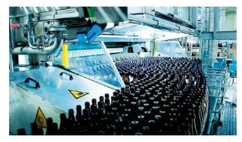
Object classification is one example of a machine vision recognition task. In this user case, new and used bottles are classified in the infeed zone at the bottlewasher machine
