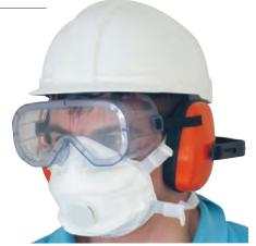
The FFP3 is suitable for use in work environments that could create high dust levels or involve silica or wood dust. Some woods are described as toxic, especially some hard woods, and respiratory protective equipment (RPE) with an APF of 20 is appropriate.
