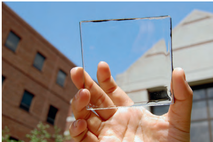
MSU doctoral student Yimu Zhao holds up a transparent luminescent solar concentrator module. Photo by Yimu Zhao.
