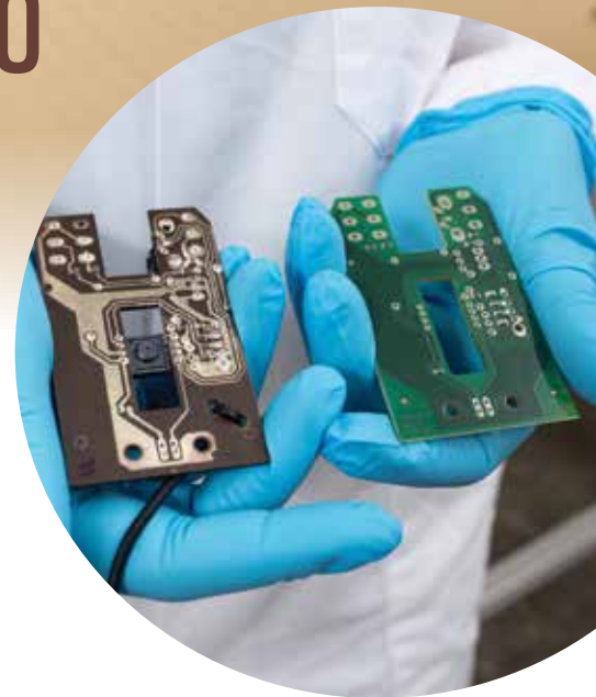
Above: The 'green' circuit board is actually not green, but brown: on the left is a mouse circuit board made of lignocellulose, on the right is a conventional mouse circuit board made of non-renewable raw materials.
