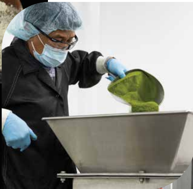
Left: Operator empties a scoop of hand-weighed powder into the mixer intake which remains stationary as the vessel turns.
