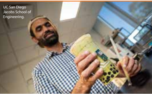
ABOVE Study co-first author Muhammad Inam Khan demonstrates fingertip placement on the sticker while gripping a boba drink. Three fingertips rest on the arched biofuel cell (left) while the tip of the middle finger rests on the vitamin C sensor (right). RIGHT Study co-first author Ryan Burns uses the sticker on a cup filled with orange juice.
