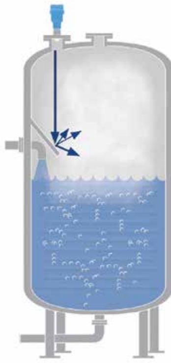
Figure 3: Deflector plates are typically installed near obstructions and angled to redirect radar waves that would otherwise reflect directly back to the transmitter. However, their installation can be challenging.
