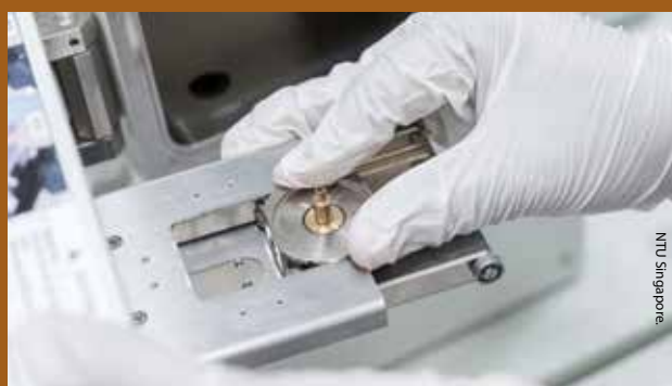
Graphite on a sample holder being loaded into a field emission scanning electron microscope for the NTU team's X-ray experiments.
