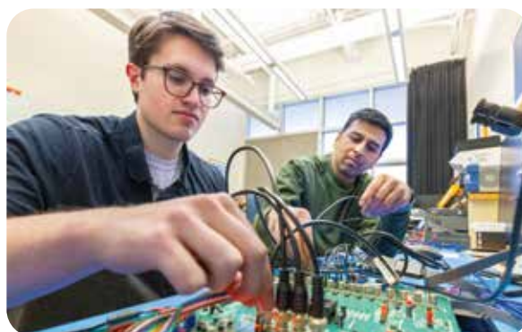
Daniel Zeznick, foreground, and Teju Das, associate professor of microelectronic engineering, test their integrated circuit on a PCB platform built in-house to assess power and control in integrated circuits.
