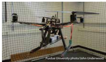
This AI-powered drone contains event-based cameras that help it to avoid obstacles and reach its programmed destination.
