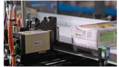
A high-resolution camera verifies the data that has just been printed in order to discard faulty products immediately. Wipotec's Traceable Quality System can be expanded with several modules, and all these functions are perfectly synchronised and can easily be controlled via a central user interface.
