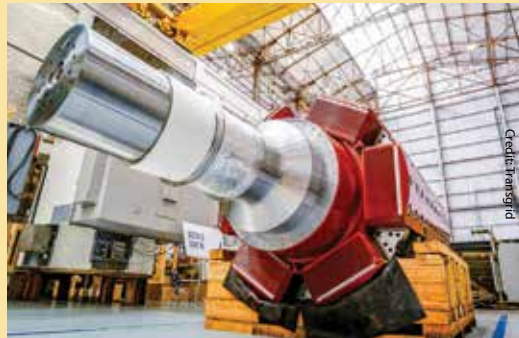
The rotor of a GE Vernova synchronous condenser.
