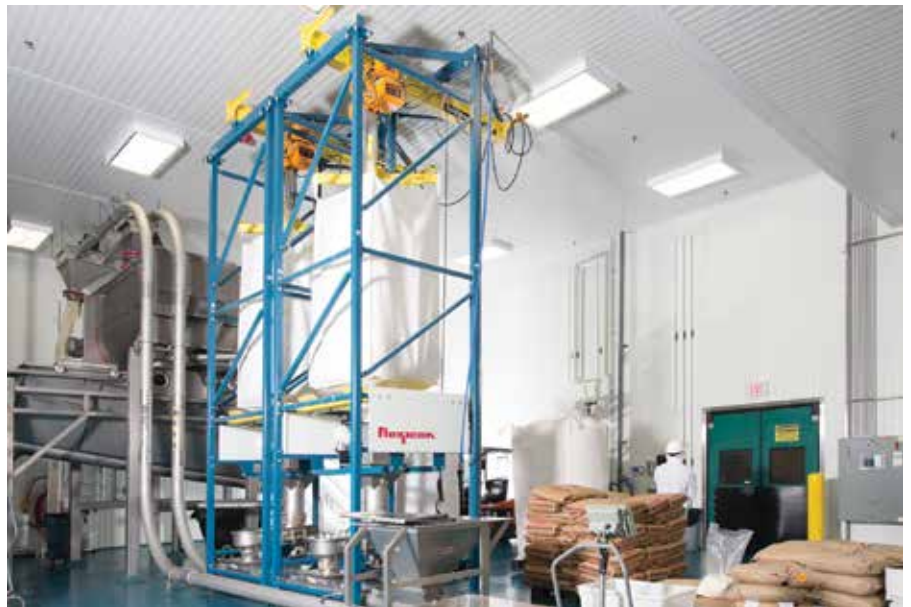
The granola tubular cable conveyor circuit: major ingredients are metered from two bulk bag dischargers into the tubular cable conveyor that feeds the mixer.
