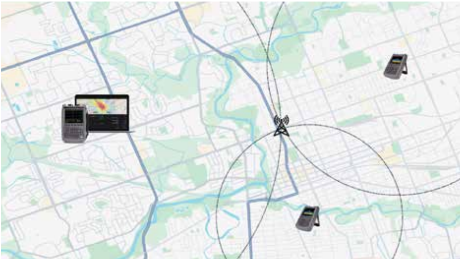
Figure 1: Distributed field measurements combined with TDoA processing enable rapid, wide-area localisation of interference sources.
