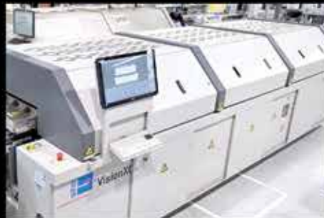
Nitrogen Enabled SMT Reflow
