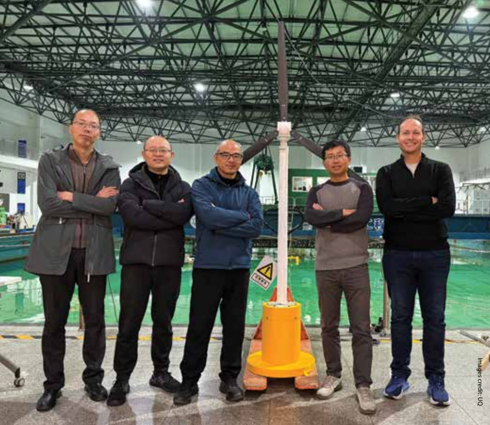
Wave basin testing showed Zhao's floating turbine model can survive a one-in-100-year storm and be moored in up to 200 metres of water.
