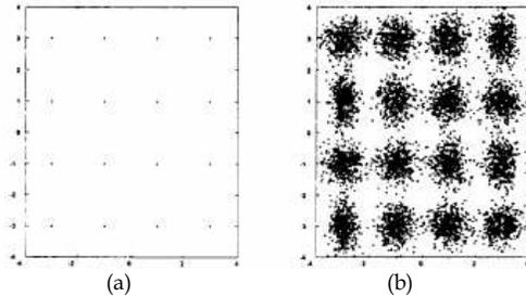
**Figure 2.** Phase noise effects on 16-QAM modulated OFDM signals (a) original 16-QAM constellations (b) 16-QAM constellations corrupted by phase noise
