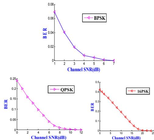
**Figure 3.** The BER vs. SNR for OFDM using BPSK, QPSK, 16PSK respectively
