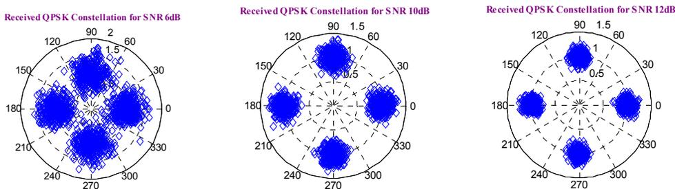
Figure 6. Received QPSK constellation for corresponding SNR values of 6dB, 10dB and 12dB
