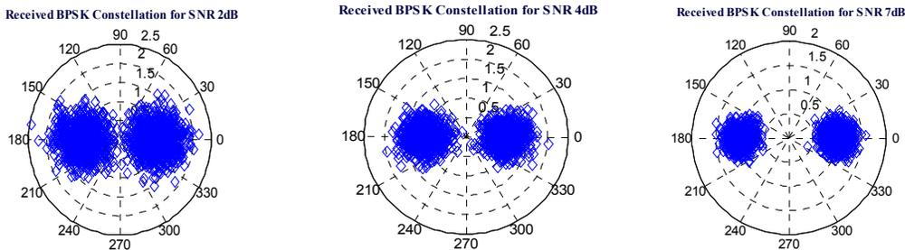
Figure 5. Received BPSK constellation for corresponding SNR values of 2dB, 4dB and 7dB
