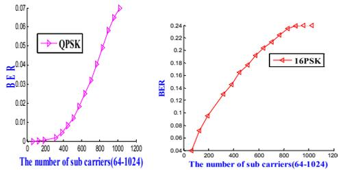
Figure 4. The number of sub-carriers vs. BER, when SNR=10dB
