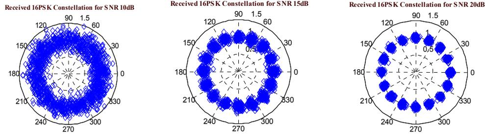
**Figure 7.** Received 16PSK constellation for corresponding SNR values of 10dB, 15dB and 20dB
