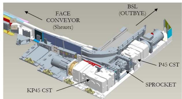
Figure 2: Typical maingate using two(2) CST Gearboxes
