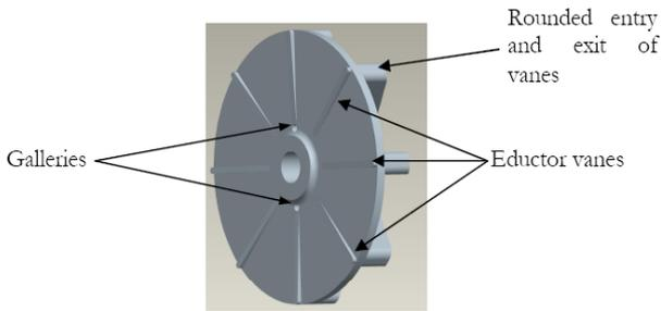
Figure 9: Features of Impeller
