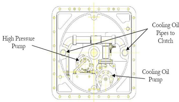
Figure 5: Supply Unit 45 CST Physical Geometry of Pump
