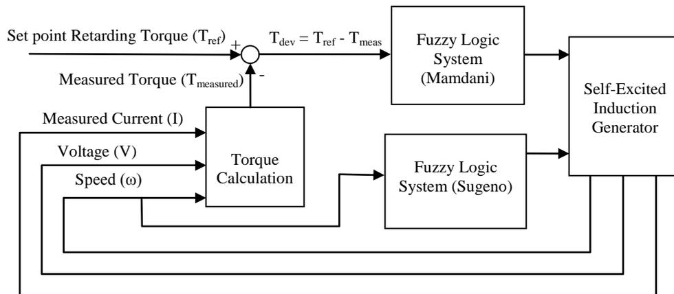
Figure 2 Control scheme of a self-excited induction generator using two fuzzy logic systems
