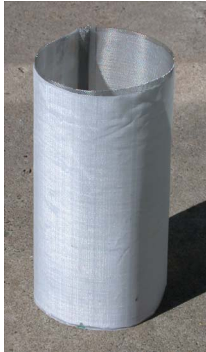
Figure 65 – ‘Pot’ for root barrier studies made of nylon root mesh and Termimesh ®
