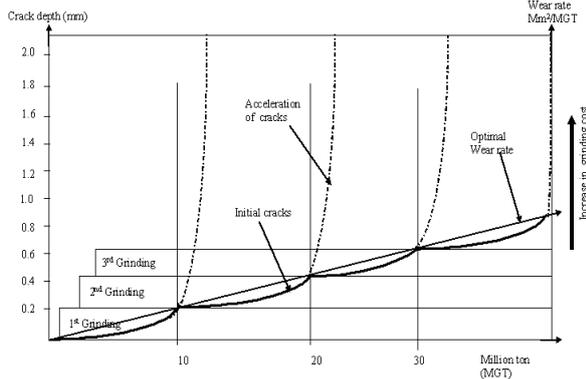
Fig 2. Achieve balanced wear by reducing cracks [14]
