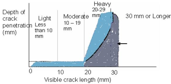
Fig 5. Visible crack length against depth of crack penetration
