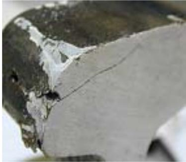
Fig 1 Rolling Contact Fatigue defect
