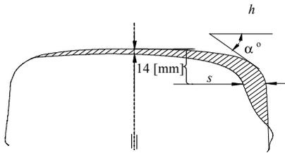
Fig 3. Central vertical wear *h* and side wear *s*
