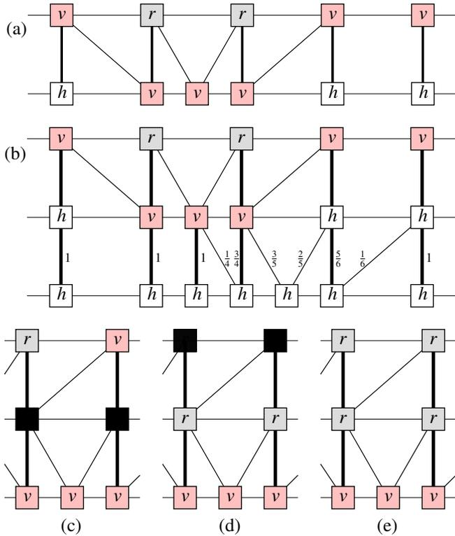
Figure 6: An example insertion. (a) Initial state. (b) Create a new layer (Step 3). (c) Mark the relevant points as *visible* (Step 4) and their parents as *to be replaced* (Step 5), shown here as a solid black square. (d) Recurse up to the next level (Steps 6, 5). (e) Final result.
