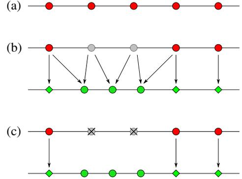
Figure A.11: (a) Row  $B$  of Figure A.10 before insertion of the new point. (b) The new point is inserted. Its position and the positions of the new points either side are calculated from the existing points (Equation 2). (c) The end result is that two *replaced* points are removed from the topmost layer and three points are made *visible* to the user from the next layer. All other points in that layer are calculated trivially from the corresponding point in the top layer.
