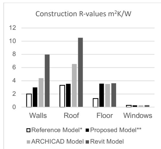
Figure 2: Construction R-value Calculations
