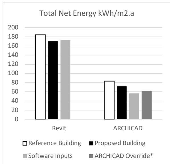
Figure 5: Whole Building simulations completed with the updated construction R-value calculations
