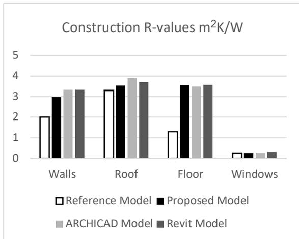
Figure 4: Updated Construction R-value calculations compared
