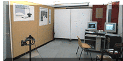
Figure 4: Set-up of Equipment: to the left, the HMD with tracking-device; to the right, the PC with communication software and image from the HMD
