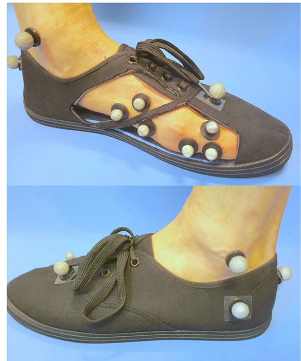
Fig. 2 Location of foot markers used for kinematic analysis. Figure from Munteanu SE, Landorf KB, McClelland JA, Roddy E, Cicuttini FM, Shiell A, Auhl M, Allan JJ, Buldt AK, Menz HB: Shoe-stiffening inserts for first metatarsophalangeal joint osteoarthritis (the SIMPLE trial): study protocol for a randomised controlled trial. Trials 2017, 18:198
