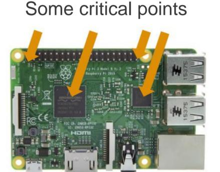
2. Computational Fluid Dynamics (CFD) simulations using ANSYS Fluent generate response surfaces relating ambient conditions to temperatures and pressures at critical points, such as the Broadcom BCM2835 CPU, mounting holes and the Ethernet controller.
