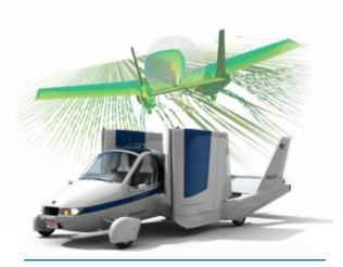
The engineering challenges that Terrafugia had to overcome in designing its innovative Transition® "flying car" were formidable. ANSYS CFD helped the team to conduct virtual airflow and wing stall speed tests, critical in advancing the project to production prototype with a high degree of confidence in the design.
