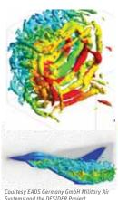
ANSYS industry experts continue to develop advanced turbulence models. Especially applicable to the aerospace industry, these ANSYS tools eliminate the trade-offs between speed and accuracy.
