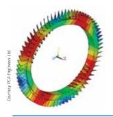
Blade flutter with compressors and turbines is a serious cause of machine failure — but until recently, design engineers were unable to satisfactorily investigate and avoid this phenomenon. Our bidirectionally coupled CFD and structural tools now predict vibration modes that occur over an entire wheel from a single-blade component model. Fluid-structure interaction accurately predicts how a design will function in a real-world environment.
