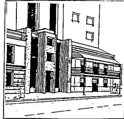
Strongly vertical proportions conflict with the predominantly horizontal streetscape
