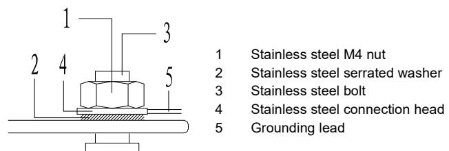
All the junctions on the conductive connection must be fixed. The fastness does not depend on soldering.
