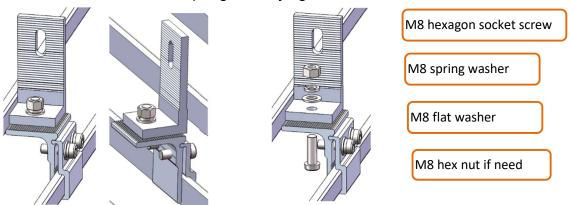
5.2.2 After fixing the L feet on the clamp, adjust the height of rail, slide the guide into the T module, and lock the bolt after adjusting location. The length of guide shall be selected according to the corresponding drawing.
