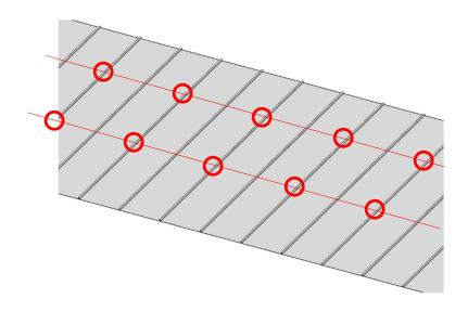
Installation of clamp: (Bolt torque value: 8~10N\*M)
