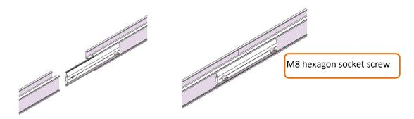
Used by TYN53、CG019、TYN28 rails etc. (External lock connection)
