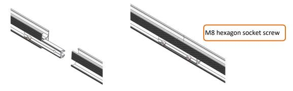
Used by CG010、TYN305、TYN355 rails etc. (Internal lock connection)
