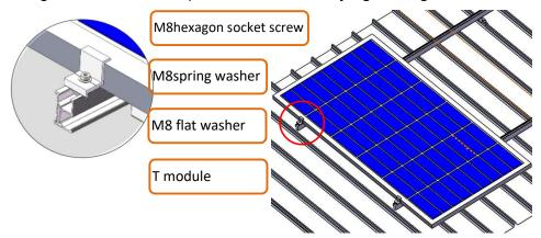
5.4.2 After first PV module installation, place the second PV module on the rail. Adjust the position and fix the first and the second module by mid clamp.
