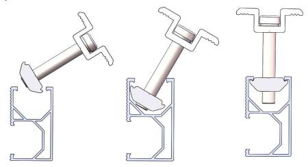
5.4.1 Place PV module on the rail and adjust position according to the drawing. Fix the end clamp with PV module by tightening the bolts.
