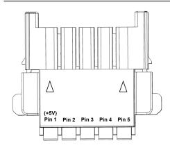
3. Connect the signal cable according to pin definition (2.2.6.1) and must connect to the Pin 1 (+5V).
