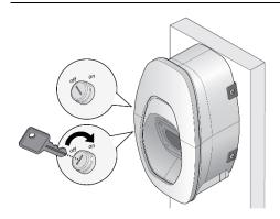
The key switch is located on the side of the product. The EVSE is authorized to charge when the key switch is in the "On" position.
