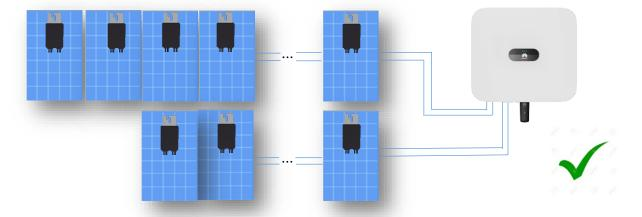
2) For SUN2000-8/10/12/15/17/20KTL-M2 inverter, it has two MPPT trackers and each tracker has two string inputs connected in parallel. Full optimizer deployment has
