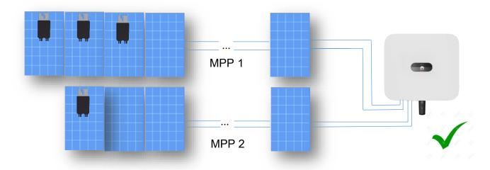
2. For SUN2000-8/10/12/15/17/20KTL-M2 inverter, inverter has two MPPT trackers and each tracker has two string input connected in parallel.
