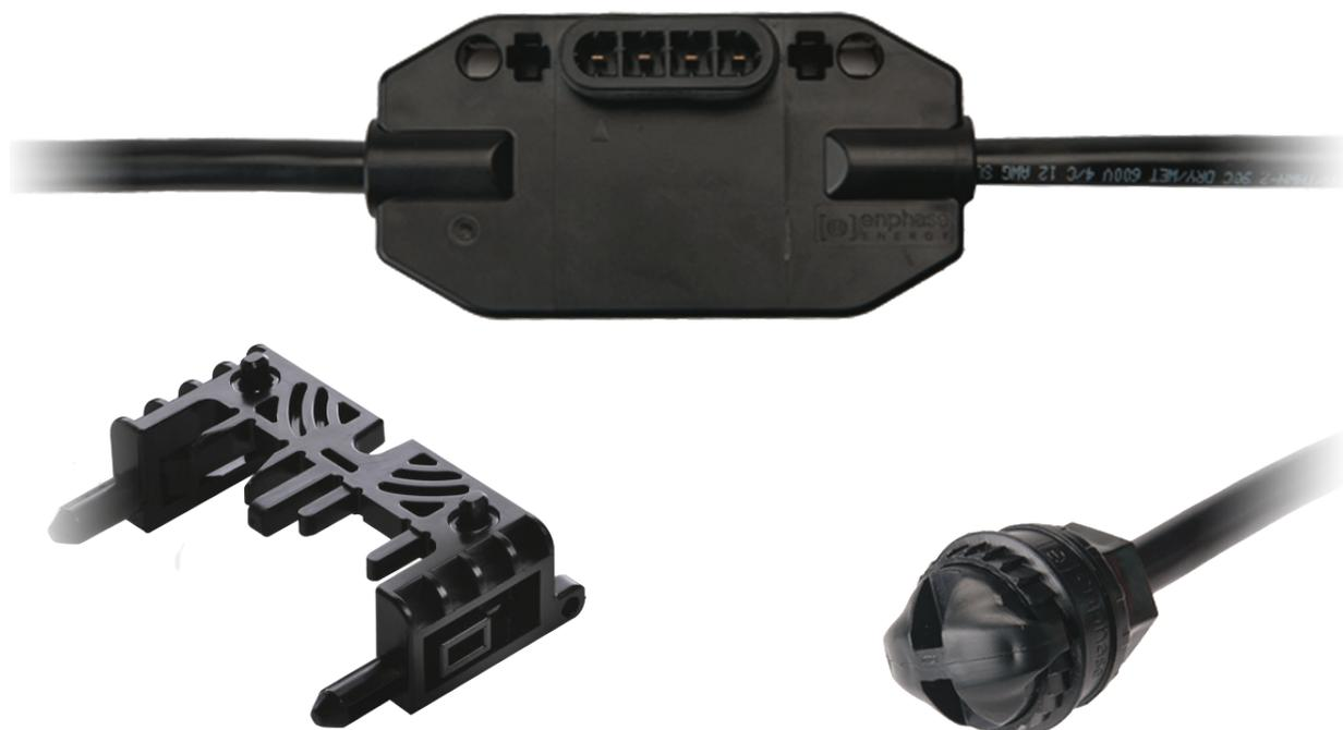
The **Engage Cable** is a continuous length of 2.5mm<sup>2</sup> cable with pre-installed connections for Enphase Microinverters. The cable is handled like standard outdoor-rated electrical wire, allowing it to be cut, spliced, and extended as needed.
