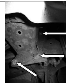
3. On 99-02 models, remove the (3) bolts attaching bumper to front of frame on either side.
