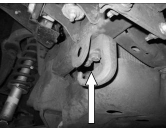
7. Remove the tow hooks & shipping lugs from the bottom of each chassis rail (retaining the tow hooks & all of the fasteners whilst discarding the shipping lugs).
