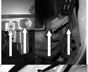
10. Remove the (2) bolts and (2) nuts on each side and remove brackets from fenders.
