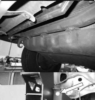
11. Remove and set aside the factory skid plate.
