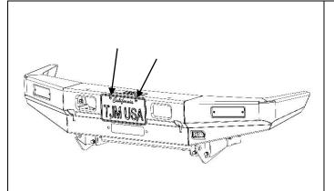
24. Using M6 x 1.0 x 16mm Button Head Bolts (2), M6 x 12mm x 1.6mm Flat Washers SS (4) & M6 Nyloc Nuts (2), secure the license-plate in place at the indicated locations.
