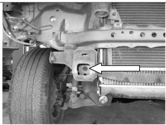
6. On 96-98 models, remove the bolt at the front of each frame horn and remove cone from frame.
