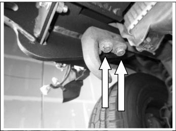
13. Place tow hook in its original position and loosely attach with bolts previously removed. Install only original bolts on opposite side.
