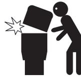
Follow all filter manufacturer's instructions. Never attempt to assemble, disassemble or adjust the filter when there is pressurized air in the system. Starting the pump while there is any pressurized air in the system can cause the filter lid to be blown off, which can cause death, serious personal injury or property damage.
