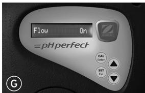
To change this function when in the "Settings" menu, enable the option list by pressing the "CAL/Enter" button (a small arrow appears on the right of the screen and the status of detection of filtration flashes). Then select "ON" or "OFF" using the "▲" and "▼" navigation buttons (G). Accept the choice by pressing the "CAL/Enter" button.
