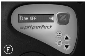
Your pH Perfect is equipped with protection to prevent over-feeding in the event there is a problem with the pH sensor, for example. The purpose of this protection, called "OFA" (Over Feed Alarm), is to pause the appliance if it has not reached the set point at the end of the time; set by default at 4 hours (F).
