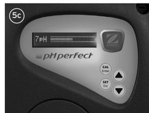
an automatic progression bar then appears (5c). Keep the sensor immersed in the buffer solution for 30 seconds.
