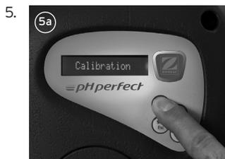
Keep the "CAL/Enter" button pressed for more than 5 seconds until "Calibration" appears on the LCD screen (5a).
