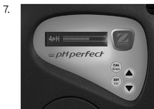
To finish calibration, press the "CAL" button. The instrument will return to measuring mode. Once the calibration is complete install the sensor in the location provided in the POD
