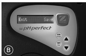
→ To exit the "Settings" menu, press the "SET/Esc" button and select "Yes" or "No", using the "▲" and "▼" navigation buttons to save the new settings or not. Accept the choice by pressing the "CAL/Enter" button (B).
