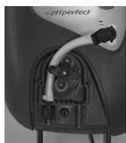
4. Position the tablet holder on "10:20" turning clockwise. Insert the left-hand connection in its housing, then pass the tube under the guide of the tablet holder. Turn the tablet holder clockwise and at the same time put the tube into the pump head up to the right-hand connection.
