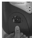
5. Replace the protective cover (place the pin in the attachment hole).
