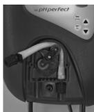
3. Fully release the left-hand connection keeping it stretched outwards, then turn the tablet holder clockwise in order to free the tube up to the right-hand connection.
