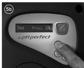
Press the "CAL/Enter" button again as indicated on the screen for calibration on pH7 (5b).
