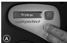
→ To access the "Settings" menu, the appliance must be ON. Simultaneously press the "CAL/Enter" and "SET/Esc" buttons for about 5 seconds until the LCD screen displays "Settings" (A).
