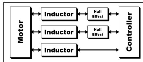
Figure 5. Motor wiring arrangement with inductors.
