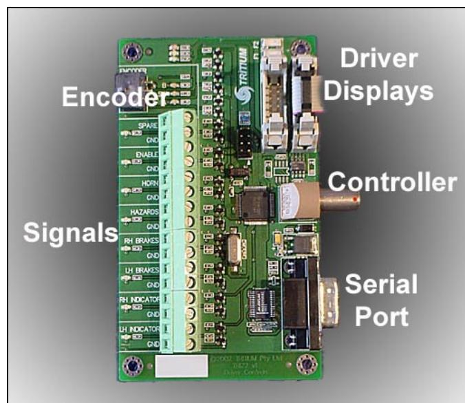
Figure 8. Connector functions of the Gold Driver Display
