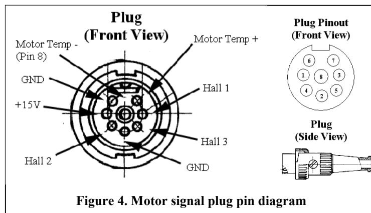
Figure 4. Motor signal plug pin diagram
